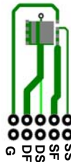
d. 120\text{ }^\circ\text{C}/\text{W} when mounted on a minimum pad of 2 oz copper
