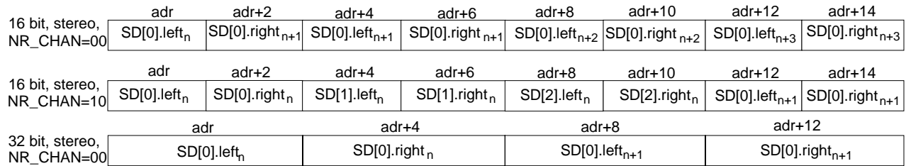
Figure 2: Examples of Audio Out Memory DMA Formats
