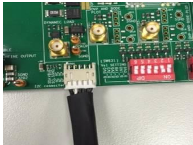
Fig. 5 – I 2 C cable connection to the evaluation board
