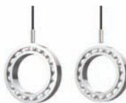
Inspecting ball bearings for foreign matter
