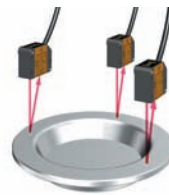
Checking the flatness of battery caps
