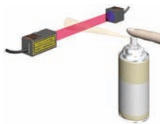
Inspecting the spray from aerosol cans
